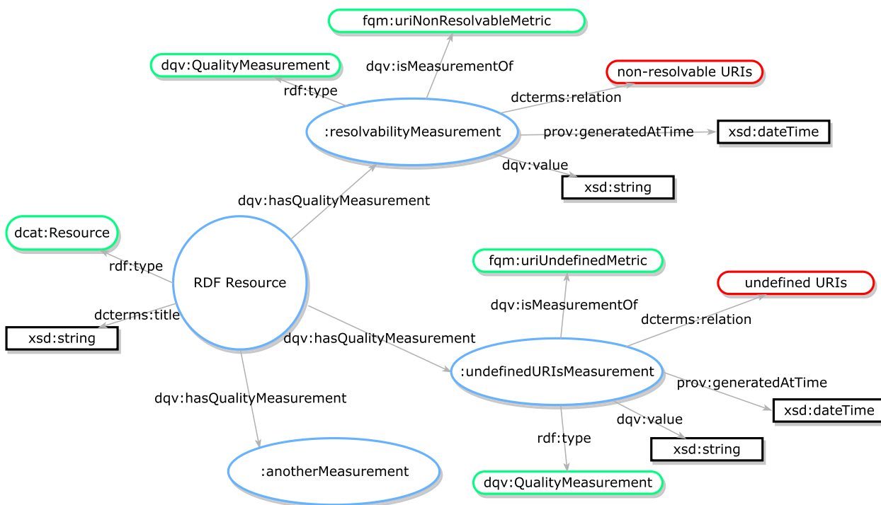
Fig. 3 The structure of an assessment report. In this model, the RDF resource is of type ‘dcat:Resource’ and connects all quality measures. Each quality measure is a node (i.e., URI) that connects its metadata, such as the metric it is measured against using ‘dqv:isMeasurementOf’, the date and time it is generated using ‘prov:generatedAtTime’, and the erroneous URIs identified using ‘dcterms:relation’. All of the node names in this diagram are examples for illustrative purposes
