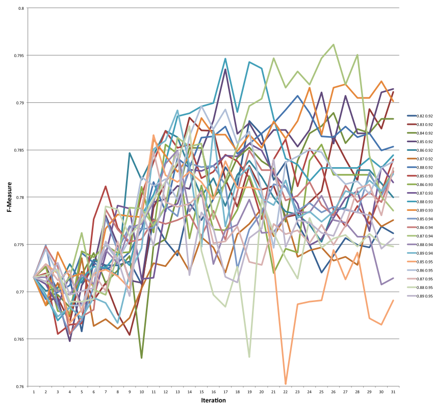
Fig. 6 F-measure values on the test set for all 22 parameter settings for 31 semi-supervised learning iterations
